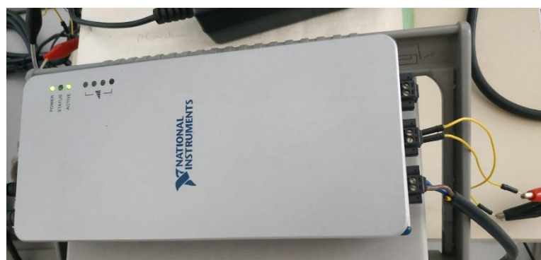
Figure 3. The NI 9225 card inside the chassis cDAQ-9191 (1-Slot, Ethernet and 802.11 Wi-Fi compact DAQ chassis) with wiring connections: Yellow wires correspond to the GPS-PPS signal while the black brings the network voltage signal directly by connecting to it with a plug.
