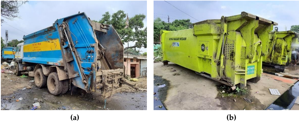
Figure 2. (a) Truck mounted refuse compactor (TMRC); (b) portable stationary compactor (PSC)
