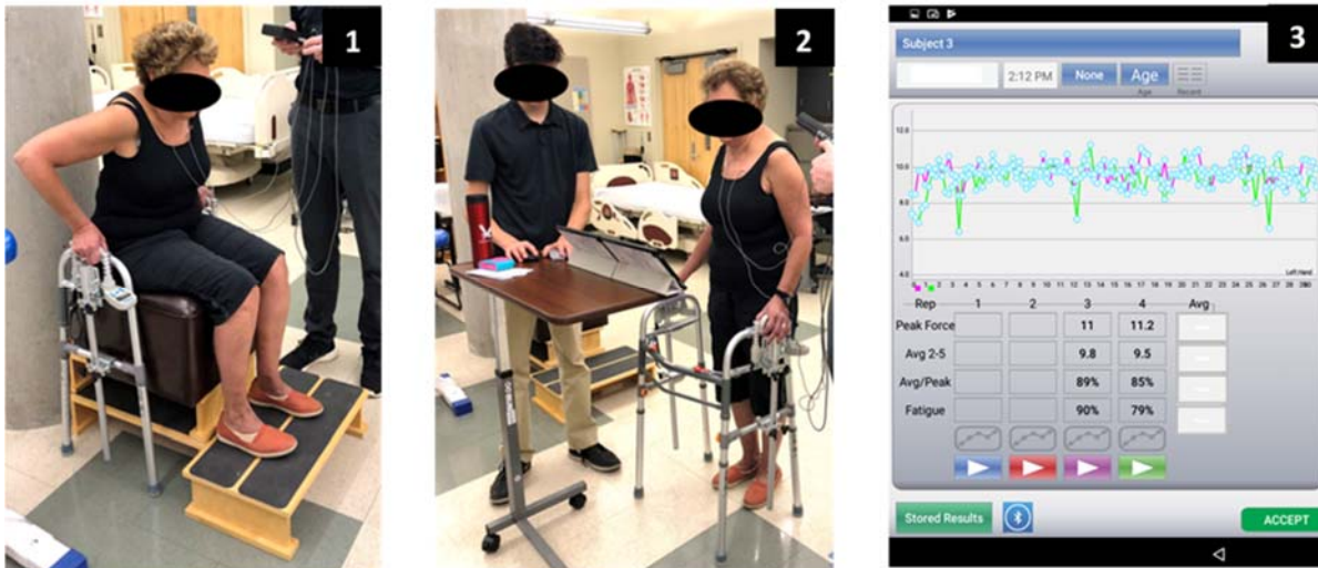
Fig. 1 Force measuring instrumentation. 1) Configuration for sit-stand transfer testing. 2) Configuration for static standing feedback training. 3) Example visual force output screen used during feedback training.
