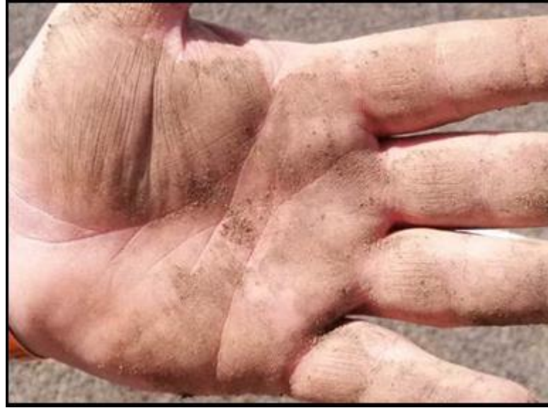
Figure 68: Demonstration of the effect of the organofunctional modification of the bitumen emulsion that is designed to adhere to granular material not contaminating the bare hand with bitumen
