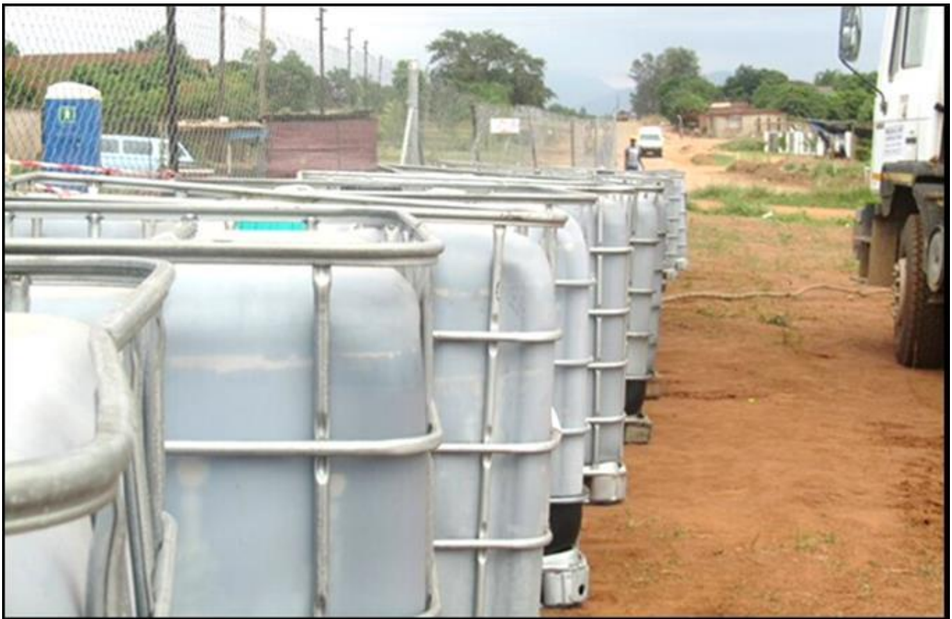
Figure 7: Flow bins containing a high-quality anionic NME stabilising agent exposed to high daily temperature conditions showing no separation or an increase in measured viscosity for periods exceeding 4 months
