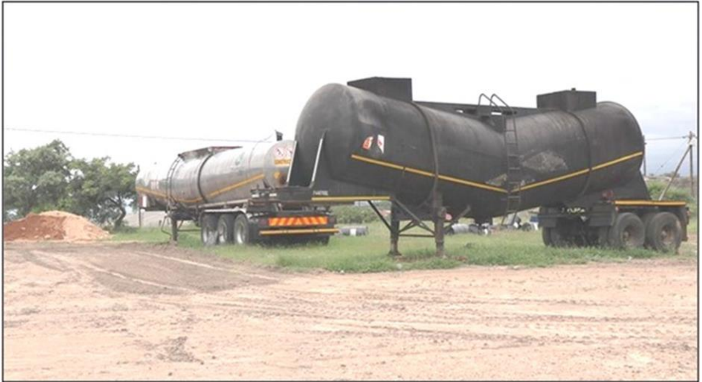
Figure 6: NME stabilising agents delivered to site in bulk storage tankers varying in size normally from 15 000 to 30 000 litres, depending on the preparation of the contractor
