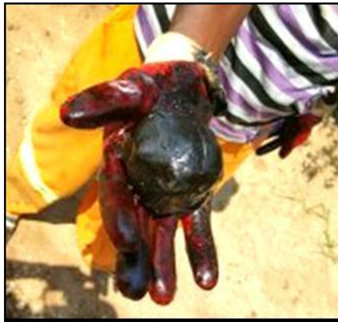
Figure 8: Typical example of an anionic NME stabilising agent that has been added to the construction water bowser containing residue from previous operations
