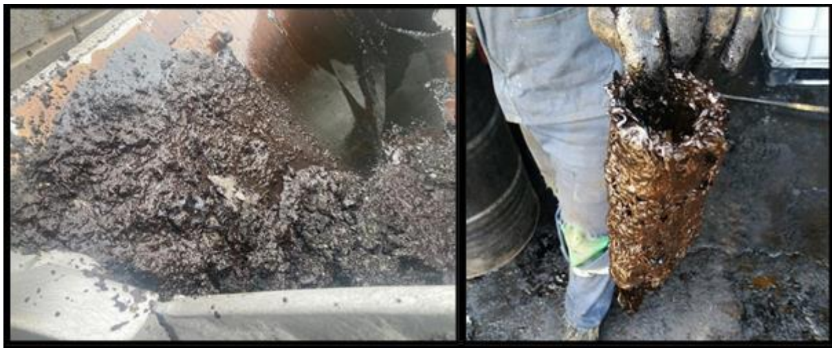
Figure 9: Typical examples of residue and state of equipment found during the pre-inspection of “clean” equipment dedicated by contractors for use for the stabilisation of granular materials using an anionic NME stabilising agent []
