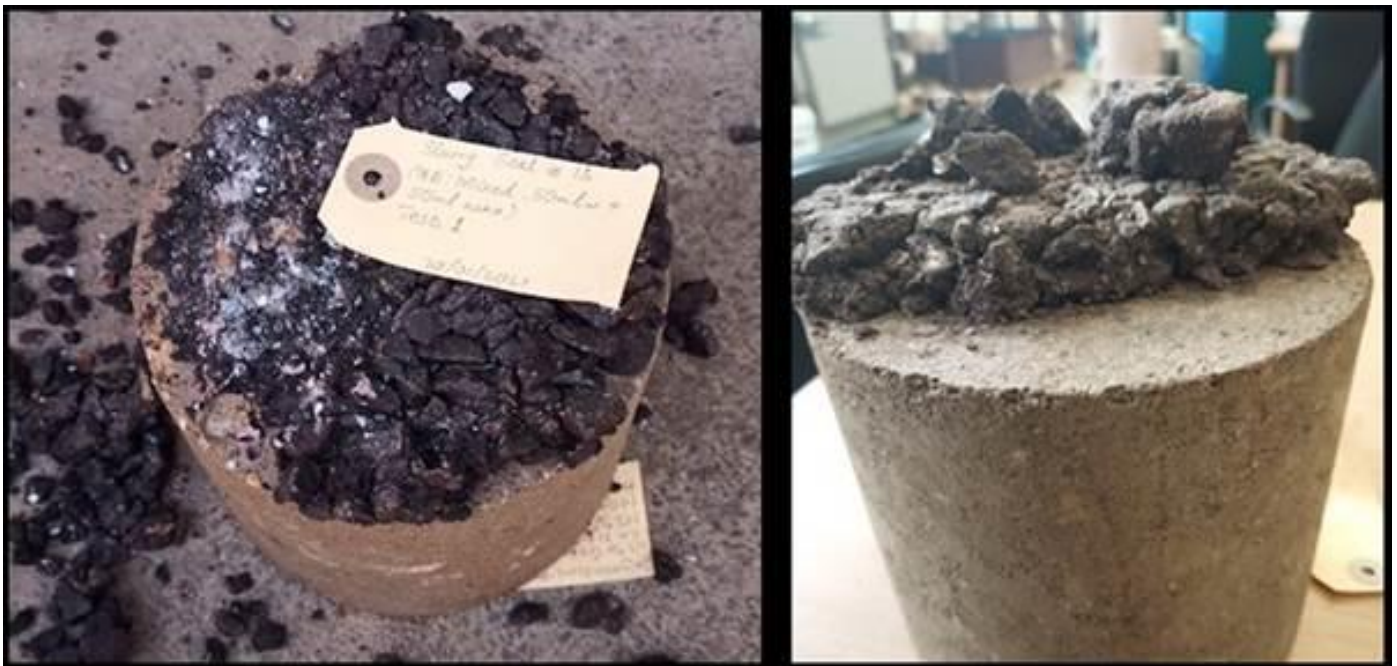
Figure 61: Application of different binders to the same NME stabilised samples showing the results of the use of compatible (left) and incompatible binders (right)
