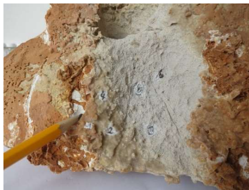
Figure 4. Rock sample with corrosion cups taken from SC Hall in Pisani Passage. Elemental composition samples were taken from seven different locations on the surface marked by pencil marks.
