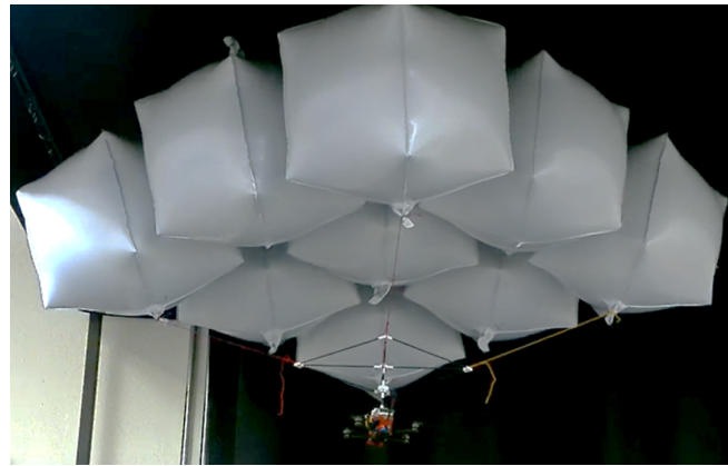
Figure 4: First prototype of the hybrid drone system using the nine off-the-shelf cubic-type balloons purchased from markets.
