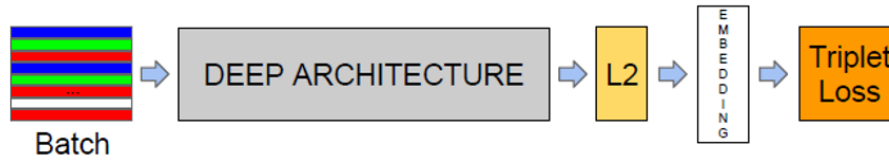
Figure 5. Face Verification Network Architecture. Adapted from [50].
