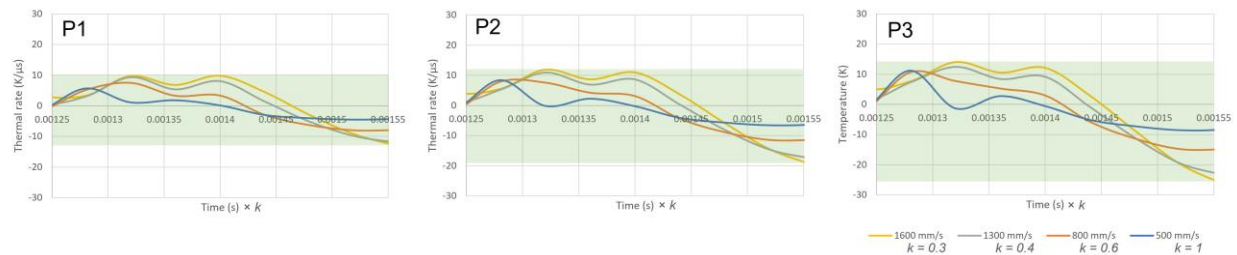
Fig 6 The effect of scan speed on the thermal rates at P1, P2, and P3 (Laser power: 100 W).
