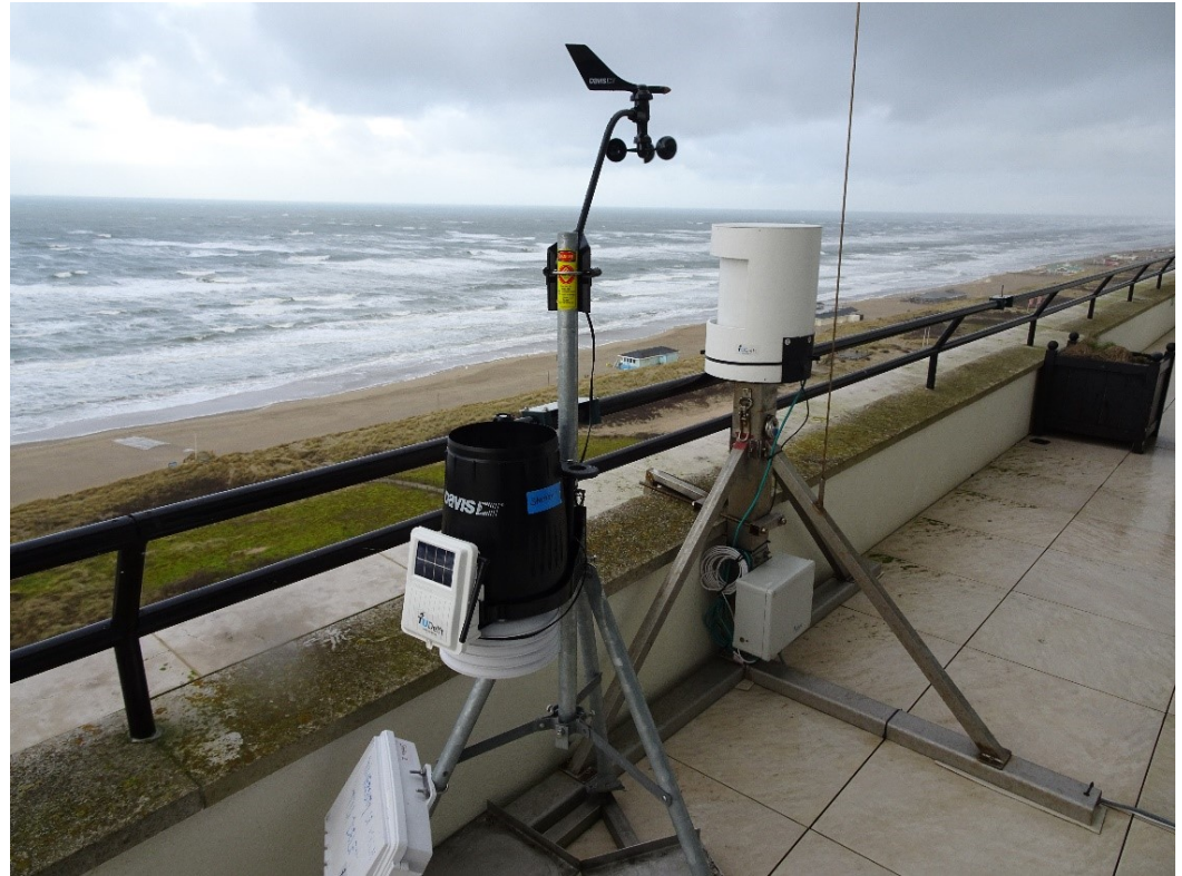
Figure 12. TLS and weather station installed on the upper balcony of the Huis ter Duin Hotel, Noordwijk, the Netherlands
