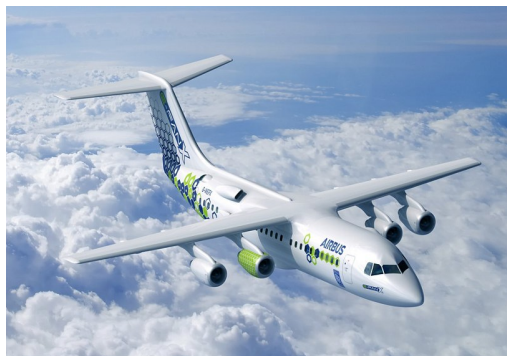
Figure 5. E-FAN X concept aircraft. The green engine was substituted by an electric motor.
