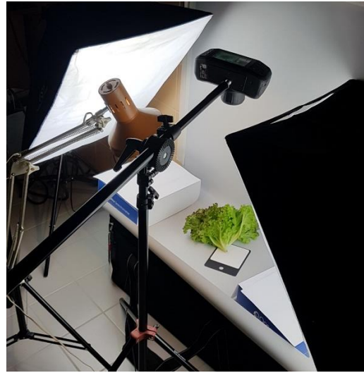
Figure 2. Hyperspectral recording of the fresh-cut lettuce leaves/plants with the SPECIM IQ camera (Spectral Images, Finland).
