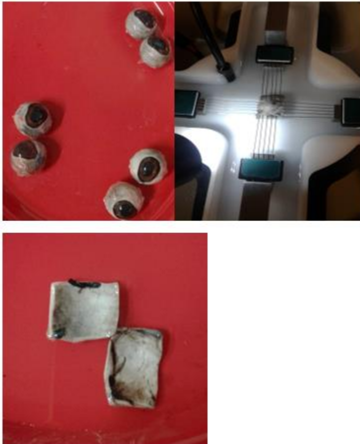
Figure 1. Experimental set-up of biaxial testing of sheep sclera soft tissue.
