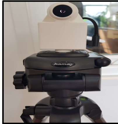
Figure 1. Thermal and Radar Sensors placed in a 3D enclosure and mounted on a tripod stand during data collection.
