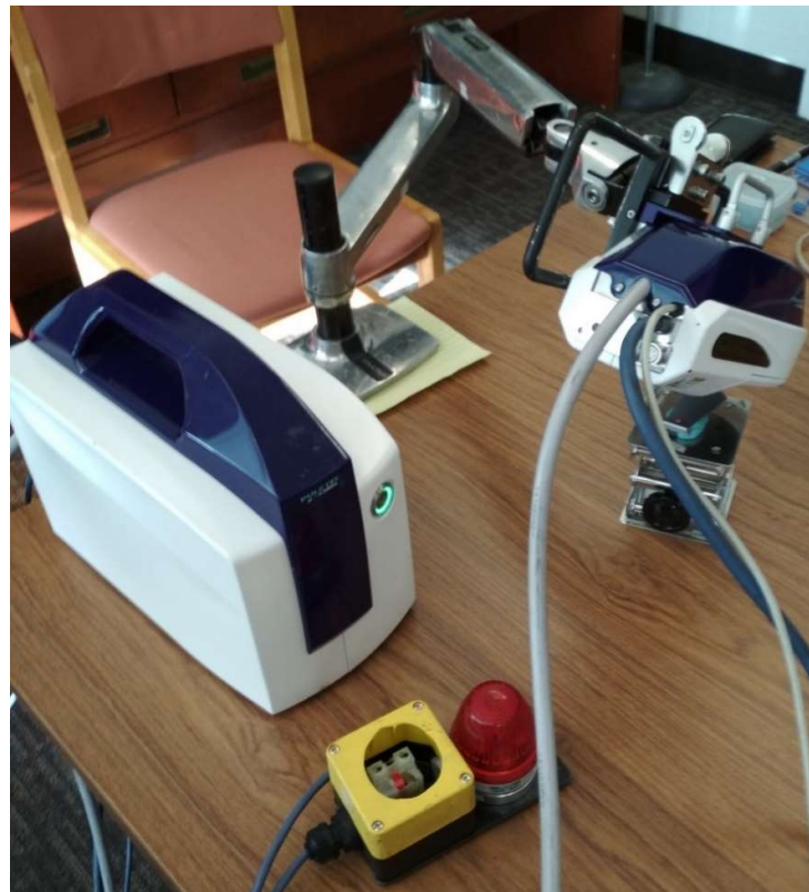
Figure 3. The experimental set-up for measuring the initial stresses on the blade surface.
