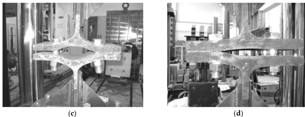
Figure 21. (a) Force-displacement curves TS HEA500; (b) Force-displacement curves TS HEB500; (c) Specimen TS HEA500 at collapse; (d) Specimen TS HEB500 at collapse. [40]
