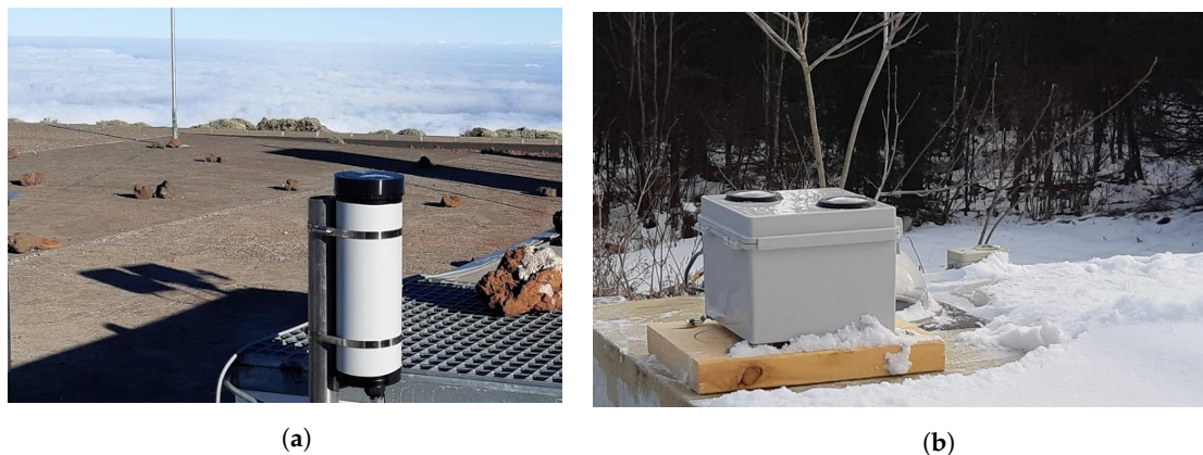
Figure 2. The CoSQM device. Panel (a) shows the version 1 of the CoSQM. That specific unit is installed at AEMET Izaña observatory (Spain). Panel (b) shows the second version of the CoSQM. This unit is installed at Saint-Camille (Canada).
