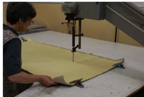
Figure 2. Cutting process of the layers for the ballistic.
