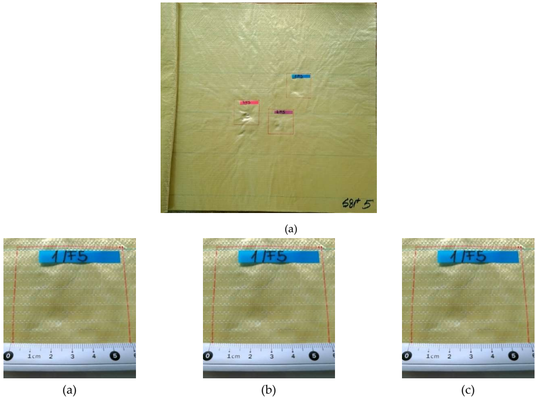
Figure 11. Frontal view of a package made of layers LFT SB1plus, (a) layer 5 (face), with details (b) fire 1, (b) fire 2, (c) fire 3.
