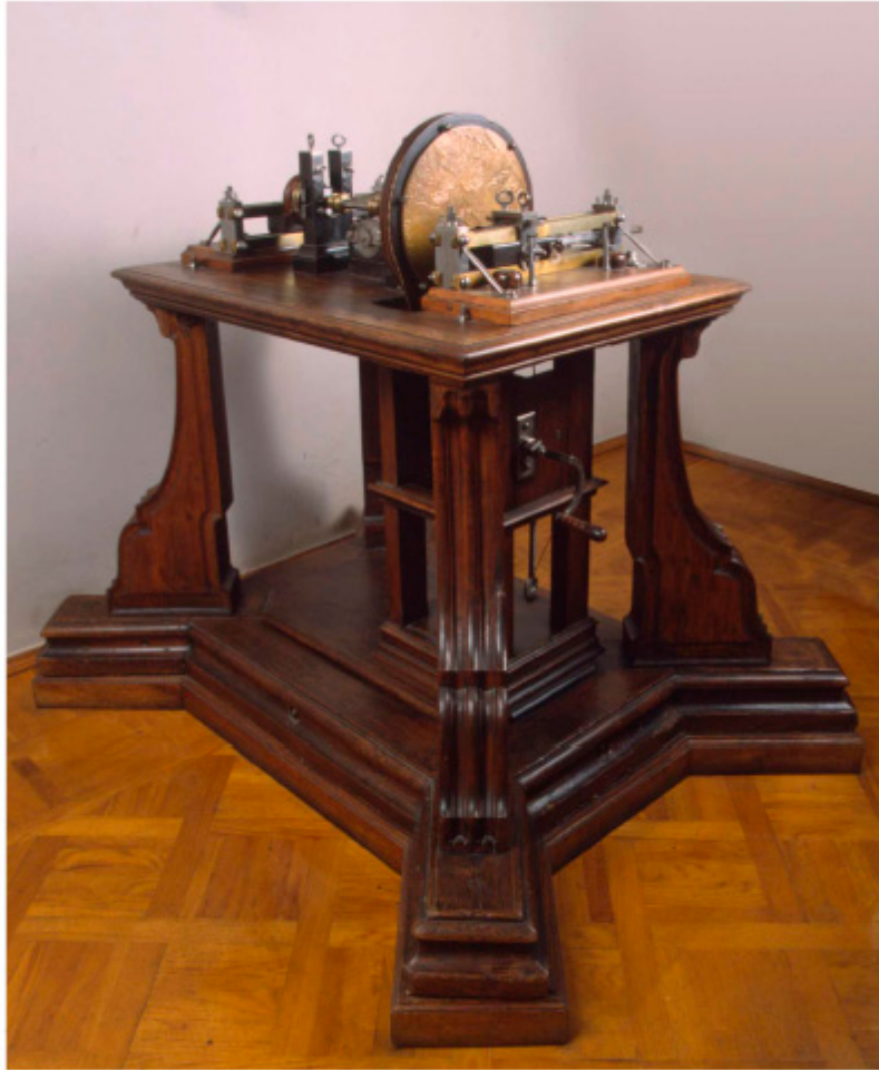
Photo. 18. The medal copying lathe by F. Singer and A. Nartov, circa 1710. The machine is intended for medal production by a large size model in automatic mode. (State Hermitage Museum, St Petersburg, www.hermitagemuseum.org ).
