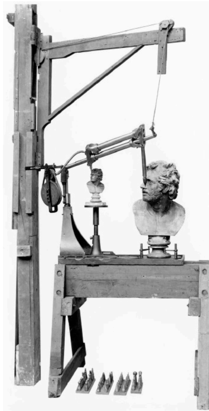
Photo. 20. 3D-pantograph designed and built by B. Cheverton, 1826. The mechanism is intended for the automatic production of reduced copies of sculptures (Science Museum, London, sciencemuseumgroup.org.uk ).
