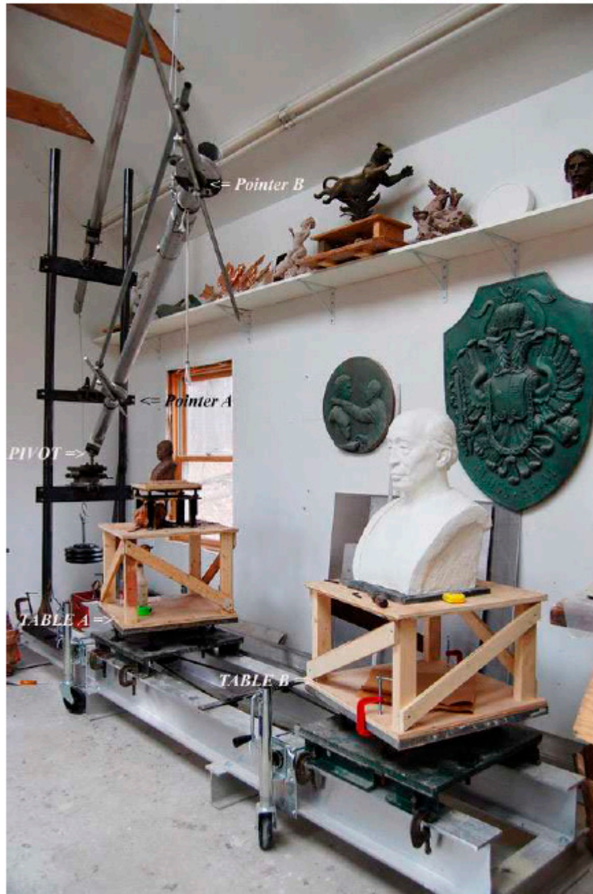
Figure 2. Modern 3D-pantograph used by sculptors (M. Keropian, www.keropiansculpture.com ). The 3D-pantograph allows to proportionally enlarge or reduce a space figure. The pantograph has a frame on which two rotary platforms are located. A model is installed on one platform (Table A), and an enlarged copy of the model is located on the other platform (Table B). A boom is attached to the frame using a ball joint (Pivot). The boom is equipped with a counterweight. There are cylindrical hinges on the boom, to which the parallelogram mechanism is attached. A sharp probe (Pointer A) is fixed on one arm of the parallelogram mechanism, a sharp pointer (Pointer B) – on the other arm. Due to a chain transmission, the platforms can be synchronously rotated around their vertical axes, putting different sides of the model/copy under the probe/pointer. If one touches the model with the probe, the pointer will show where the corresponding point of the enlarged copy is located in the space.
