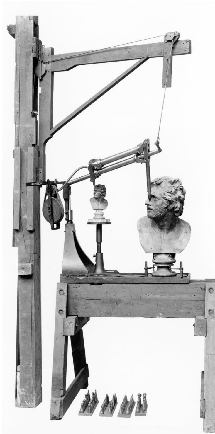
Photo. 20. 3D-pantograph designed and built by B. Cheverton, 1826. The mechanism is intended for the automatic production of reduced copies of sculptures (Science Museum, London, sciencemuseumgroup.org.uk ).
