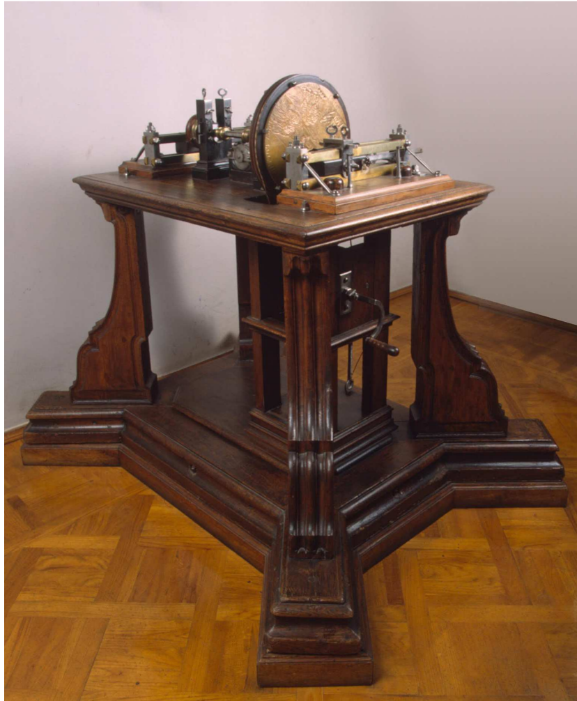
Photo. 18. The medal copying lathe by F. Singer and A. Nartov, circa 1710. The machine is intended for medal production by a model in automatic mode. (State Hermitage Museum, St Petersburg, www.hermitagemuseum.org ).
