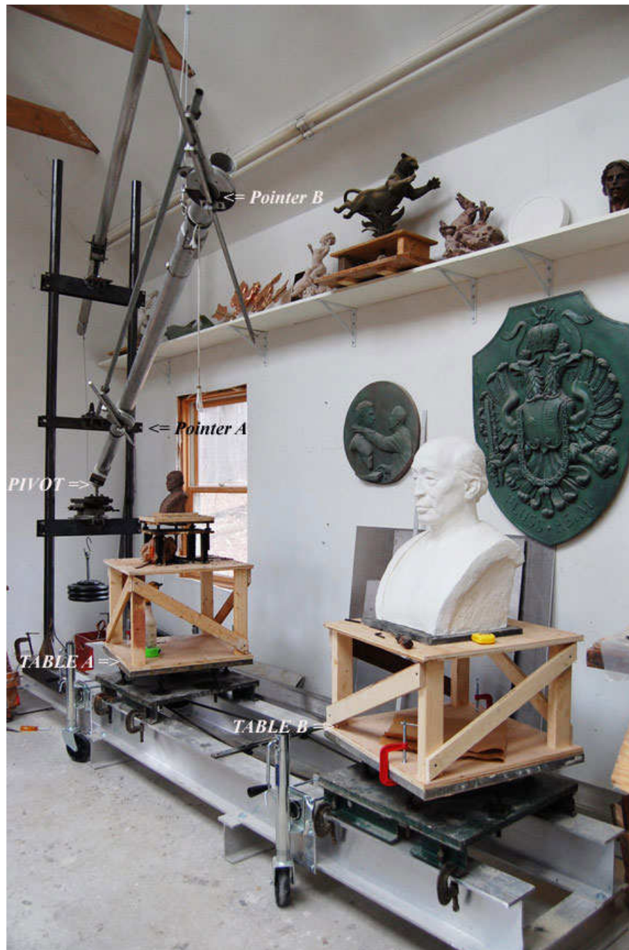
Fig. 2. Modern 3D-pantograph (photo by M. Keropian)
