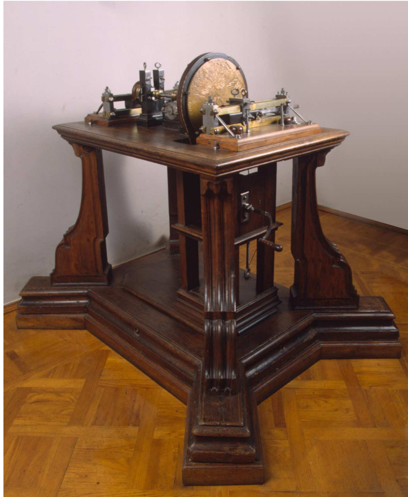
Photo. 20. The medal copying lathe by F. Singer and A. Nartov, circa 1710. The machine is intended for medal production by a large size model in automatic mode. (State Hermitage Museum, St Petersburg, www.hermitagemuseum.org ).
