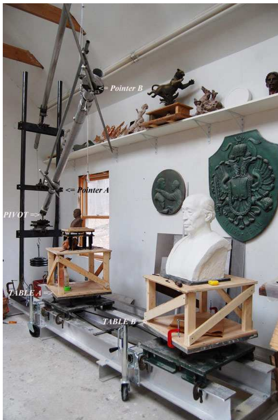
Fig. 2. Modern 3D-pantograph used by sculptors (M. Keropian, www.keropiansculpture.com ). The 3D-pantograph allows to proportionally enlarge or reduce a space figure. The pantograph has a frame on which two rotary platforms are located. A model is installed on one platform (Table A), and an enlarged copy of the model is located on the other platform (Table B). A boom is attached to the frame using a ball joint (Pivot). The boom is equipped with a counterweight. There are cylindrical hinges on the boom, to which the parallelogram mechanism is attached. A sharp probe (Pointer A) is fixed on one arm of the parallelogram mechanism, a sharp pointer (Pointer B) – on the other arm. Due to a chain transmission, the platforms can be synchronously rotated around their vertical axes, putting different sides of the model/copy under the probe/pointer. If one touches the model with the probe, the pointer will show where the corresponding point of the enlarged copy is located in the space.
