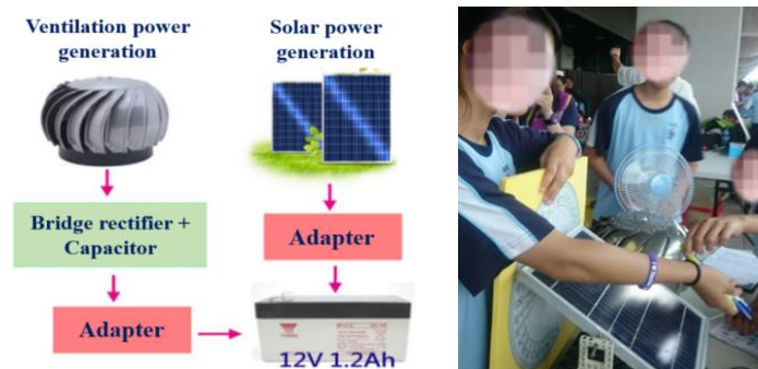
Figure 10. Flowchart and actual test of parallel power generation between ventilation generator and solar panel in the campus ( S_A-A_8-Y_6 ).
