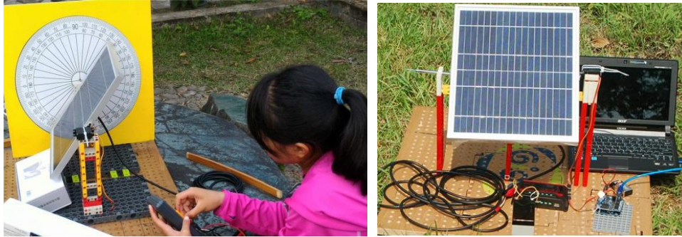
Figure 9. Students measured the angle between the solar panel and the sun, using Arduino control to obtain the best storage value ( S_A-A_3-Y_6 ).
