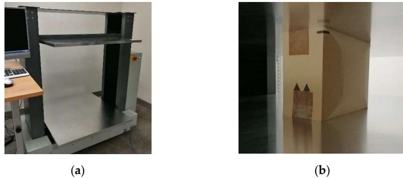
Figure 3. BCT tests: (a) BCT press; (b) packaging with the shifted offsets on the flaps.
