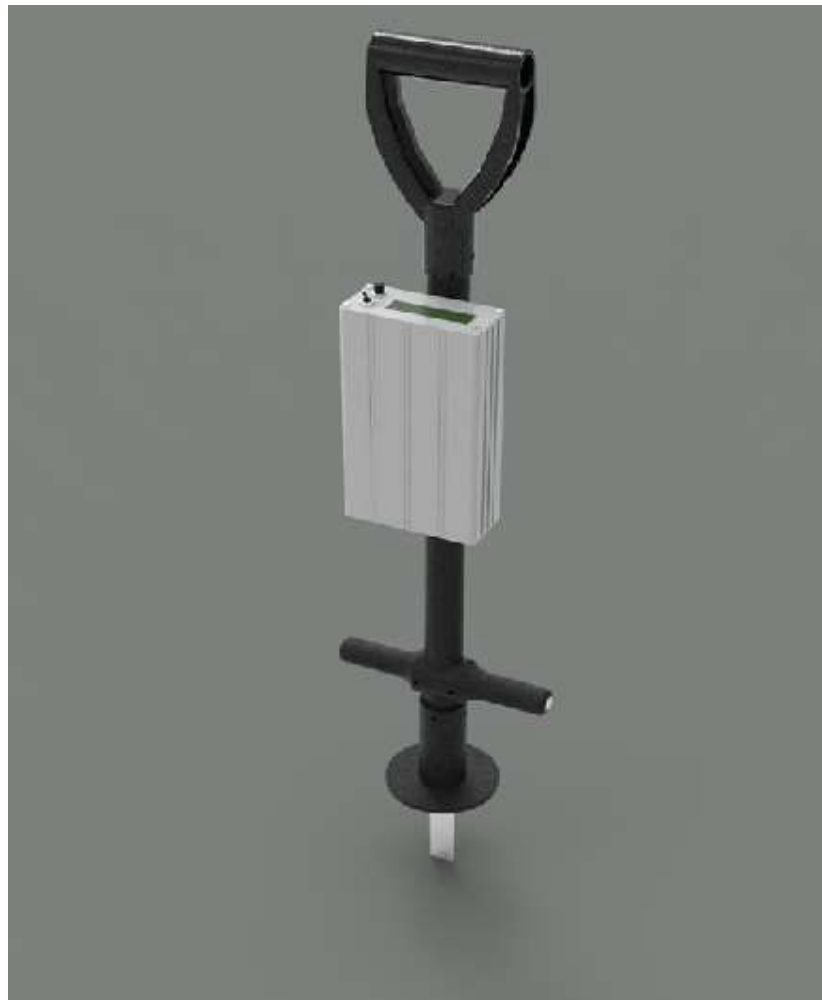
Figure 4. Two Axis Commercial Strain-gauge Sensor Probe (Going Stick)
