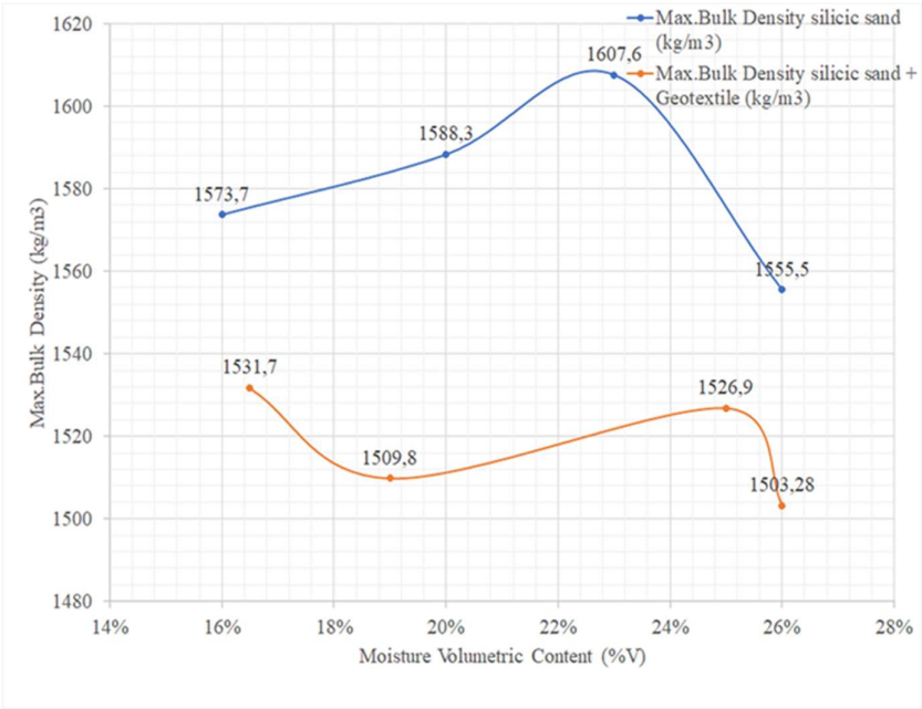
Figure 2. Bulk density of silicic sand and silicic sand and geotextile addition (2 kg/m²) with volumetric moisture content (kg/m³).
