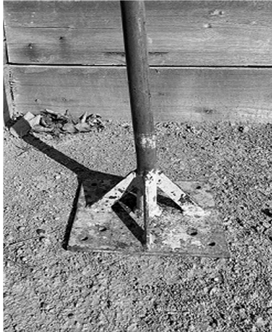
Figure 3. Image of the rammer, 4 kg mass dropped three times from a height of 0,30 m onto an area of 0,20m by 0,17m.
