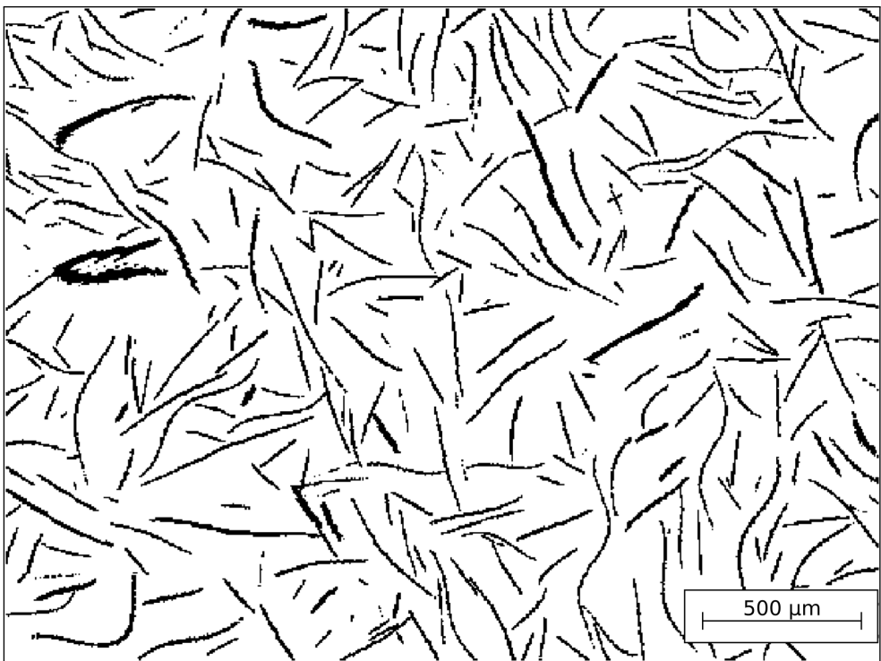
Figure 2. “Micrograph” of a synthetically generated GG-15 material, with a graphite volume fraction of 10 v. – %.
