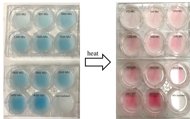
Figure 3- PDA-RTV gel. Left: Each well was irradiated with a 6 MV beam by different monitor unit doses; right: the sample after heating and curing the gel to obtain transparency.
