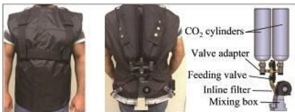
Figure 6. The air treatment system of the cooling garment with front view and back view. The prototype is composed of three parts: the layers forming the garment, the air treatment system, and the distribution channels. Reproduced with the permission. [228] Copyright 2019, Springer Nature.
