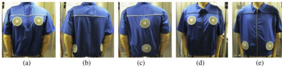
Figure 3. Small fans and openings on ventilated jacket located at different torso sites. The both fans are placed at (a) the upper back; (b) the lower back; (c) the mid back; (d) the chest (upper front); (e) the belly (lower front). Reproduced with permission. [229] copyright 2013 Elsevier.
