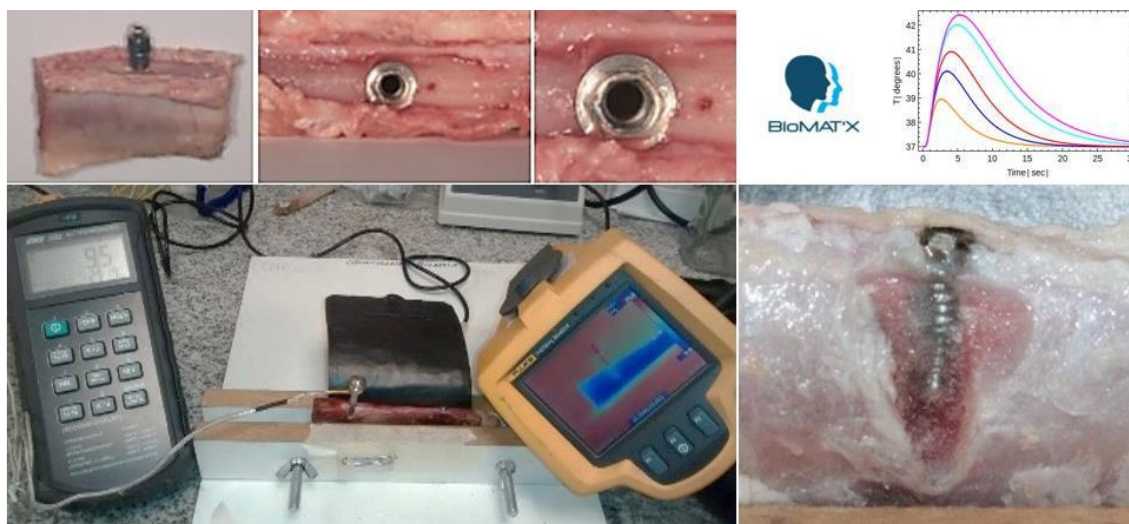
FIG. 2: Experimental Set-up; developed in-House as an ex-vivo heat distribution model employing human patient-grade titanium dental implants placed into porcine ribs (without coolant) and thermal changes monitored/recorded (quantified) using a CorDEX TP3R ToughPix DigiTherm Digital Thermal Camera.
