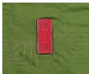
Figure.4 Integration and connection of microelectronics on textile substrate by embroidery. reproduced with permission from Taylor & Francis with order no. 501617555,[61].
