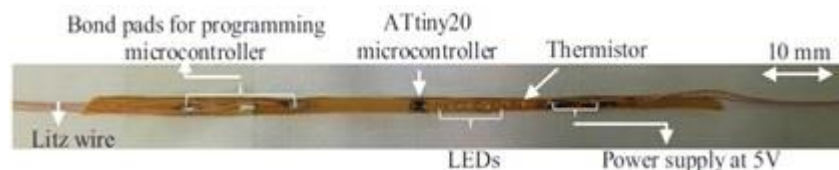
Figure 14. Direct die to wire connection reproduced with permission from advanced Material Technology, creative common attributes , https://creativecommons.org/licenses/by/4.0/ [186].
