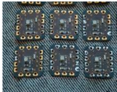
Figure 6. Hybrid solder and stiches of electronics on to textile, reproduced with permission from permission from Elsevier, with license no.4960250896870, [62].
