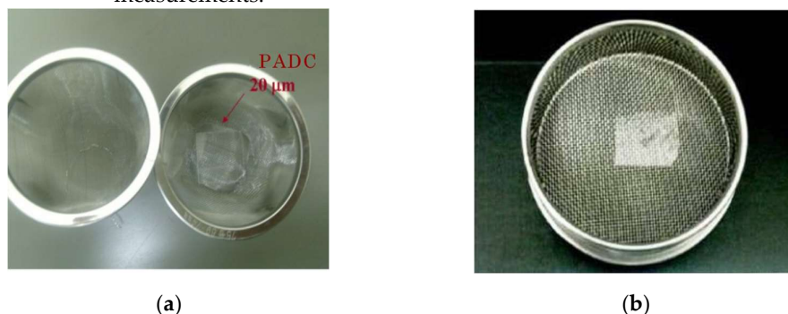
Figure 2. Photographs of PADC films during the thinning processes by chemical etching. The size of PADC films is 20 x 20 mm 2 . (a) PADC film with a thickness of 20 \mu\text{m} on stainless sieve, in the second step; (b) PADC film with a thickness of 20 \mu\text{m} in the final stage of etching on a stainless sieve with a flat base [12].
