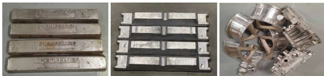
Figure 1: The different aluminium raw materials and its format used for the experimentation: a) Primary AlSi10MnMg ingots; b) secondary AlSi10MnMg(Fe) ingots; c) returns for secondary AlSi10MnMg(Fe) preparation.
