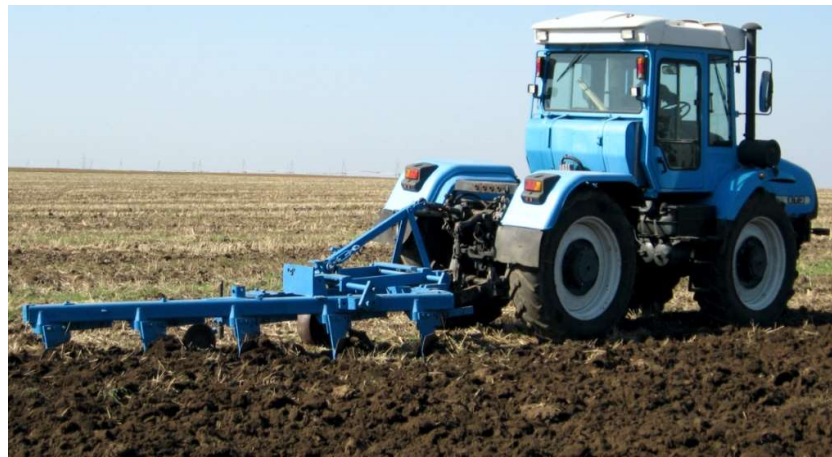
Figure 3. Tractor HTZ-17021 with five-furrow plow
