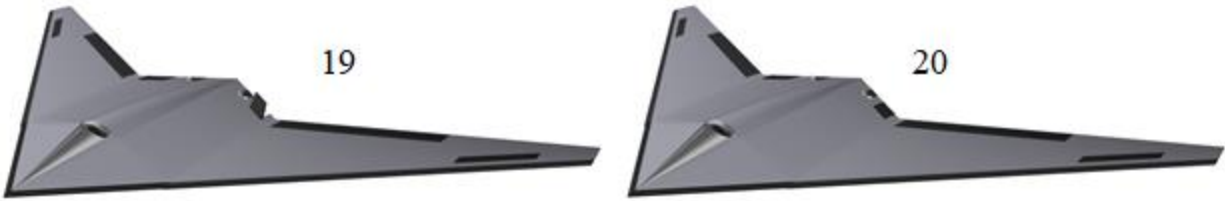
Figure 19: When the left side split drag rudder is in 60° position
