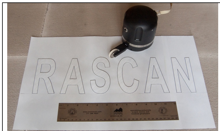
Fig. 5 Paper sheet with aluminum foil letters (ruler is 12 inches or 30.48 cm).
