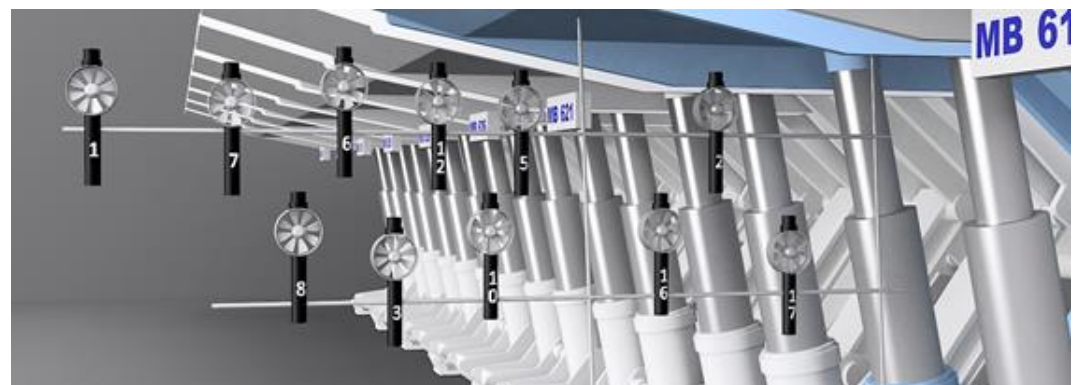
Figure 6. Location of additional sensors and the multi-point system in longwall Cw-4
