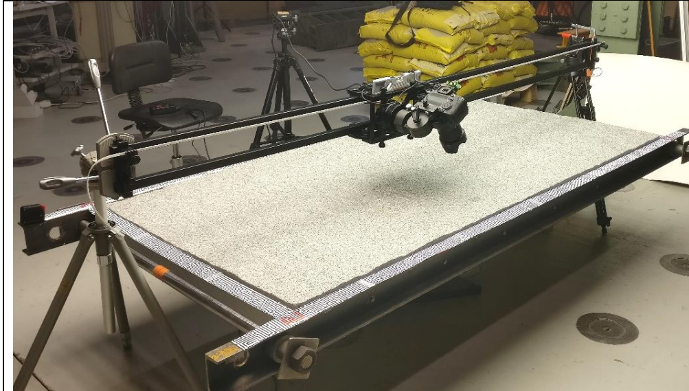
Fig. 2 The photogrammetry setup with (a) camera positioning in the back-and-forth photographing direction, (b) the slider track setup.
