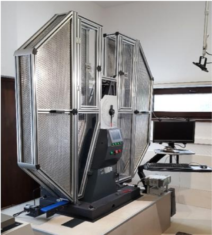
Figure 5. Instrumented Charpy pendulum used to conduct the tests.
