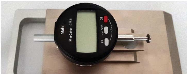
Figure 6. Measurement device used to measure the longitudinal expansion LE .
