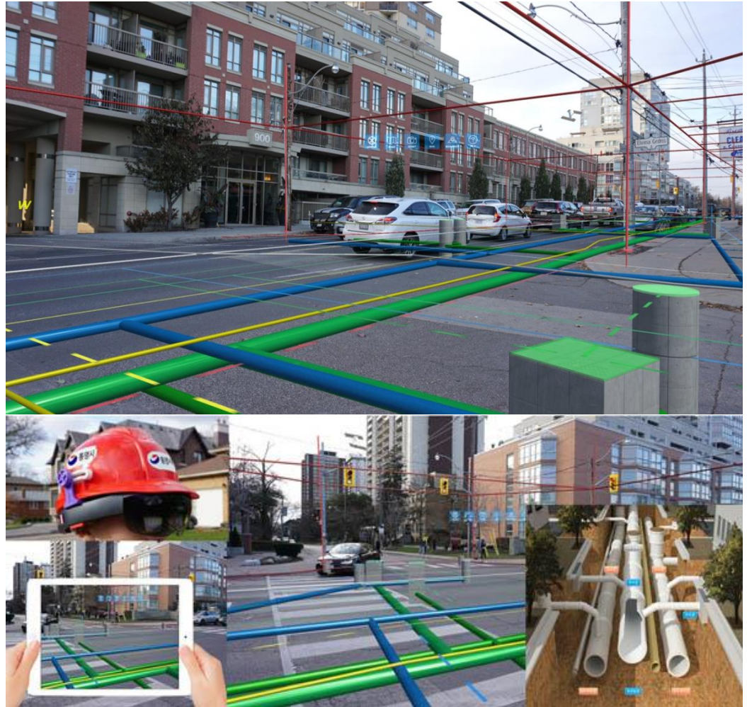
Figure 3. VGIS app view (Meemim/Up), AR technology-based underground pipeline view (Chahoo/Down)
