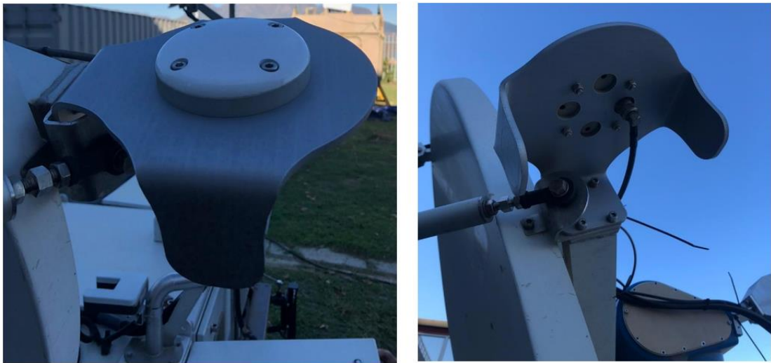
Figure 3: GPS antennas mounted on the MSR antenna. (Advance Navigation, 2017).
