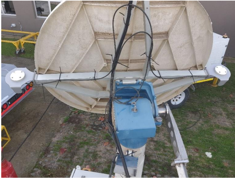
Figure 4: Antennas installed on the MSR with a baseline of 1m
