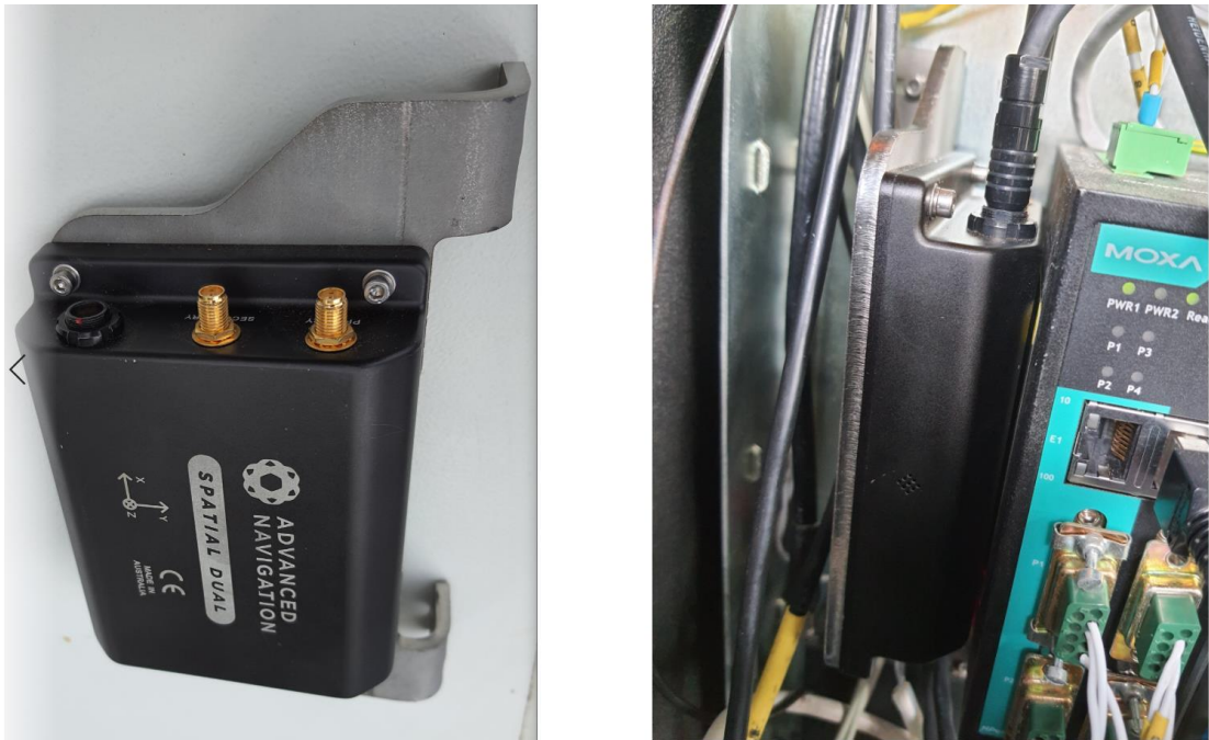
Figure 2: GPS mounted on a bracket (Left picture) and installed on the MSR (Right picture). b. Antenna mounting
