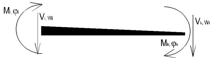
Figure 7. Sign convention for moments, shear forces, displacements, and rotations for the stiffness matrix.
