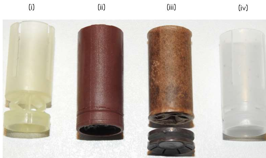
Figure 2. Wads made from biodegradable materials are available at the European market and selected for testing of biodegradability: (i) PVAL, (ii) PHA, and (iii) fiber with a liner. Also shown is (iv) a traditional wad made from LDPE. All originate from shotgun cartridges caliber 12/70 (the most commonly used).
