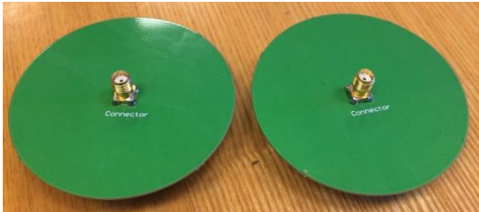
Figure 20. Two manufactured disc antennas providing the surface wave excitation.
