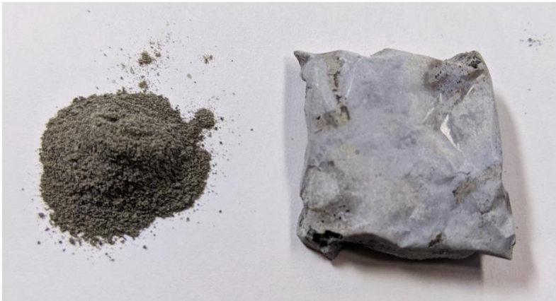
Appendix Fig. 4 A solid made from simulated sand of the moon (The sand is supplied from NICHIREKI CO.,LTD., Tokyo, Japan)
