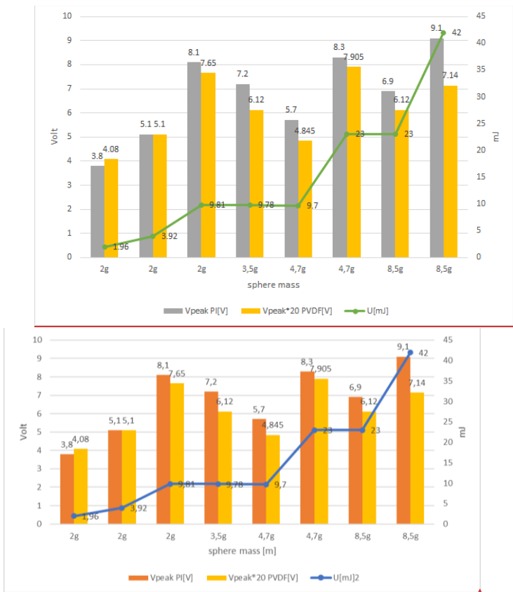
Figure 3 - Peak voltages from impacts generated by steel balls with mass ranging from 2g to 8.5g in free-fall on the aluminum laminate. The sensitivity of the two different sensors (see Figure 2) sensitivity can be compared by the output voltages: the PVDF sensor amplitudes are multiplied by a constant factor 20 to be compared with the trend of the PZT amplitude. We can observe the good correlation between impact energy and the output voltage.
