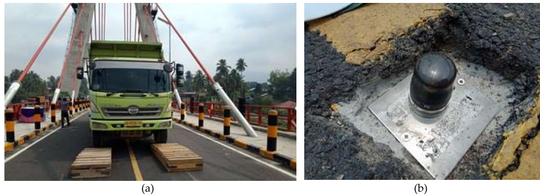
Figure 9. (a) The execution of dynamic load test; (b) The placement of accelerometer
