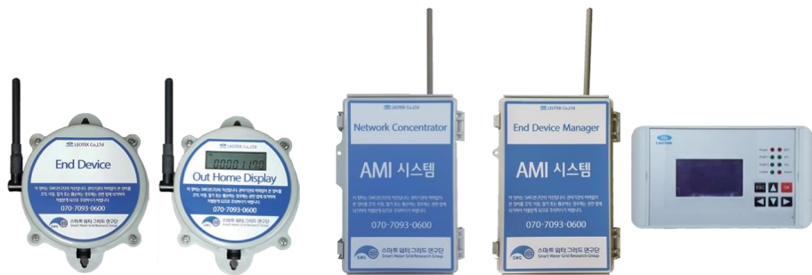
Figure 6. Developed AMI network device (SWM, OHD, NC, EDM).
