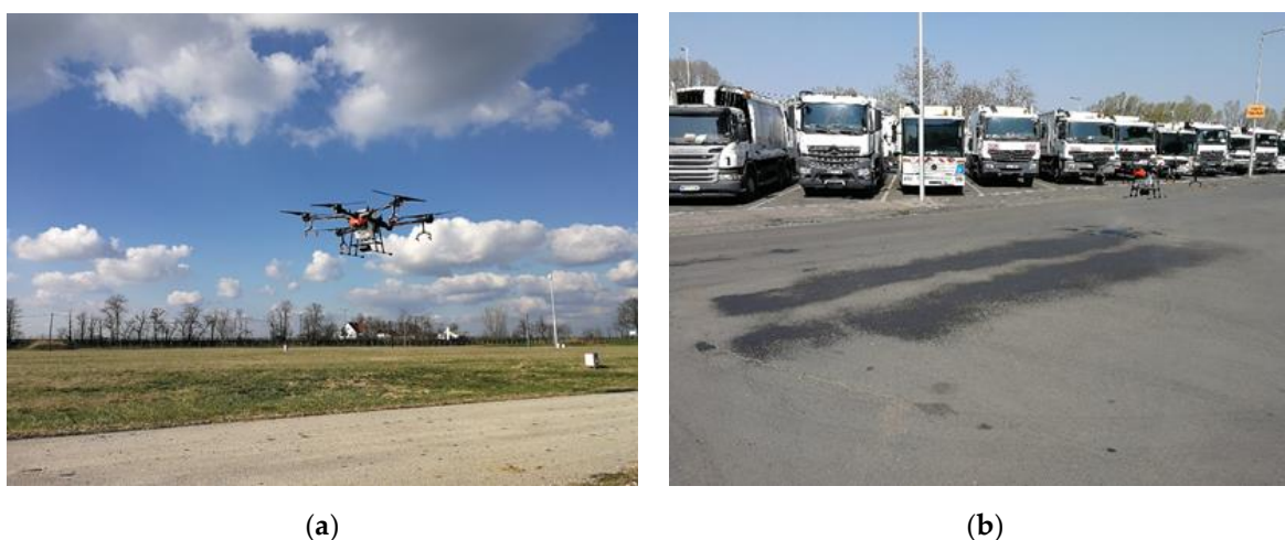
Figure 1. Agriculture drone (DJI Agras T16) using for disinfectant release test: (a) flight test at open area to calibrate the flight parameters and fluid flow; (b) footprint test in place where drone spray disinfection was required. Source: authors' archive.
