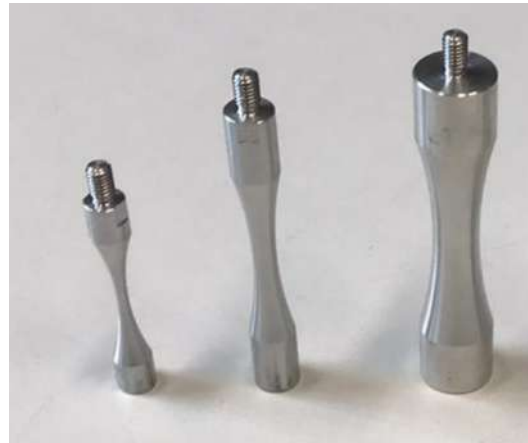
Figure 2. The three different investigated hourglass-specimens.
