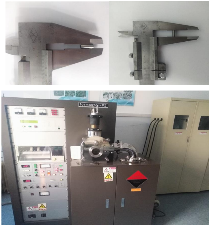
Fig. 3-Thermal expansion apparatus and sample size
