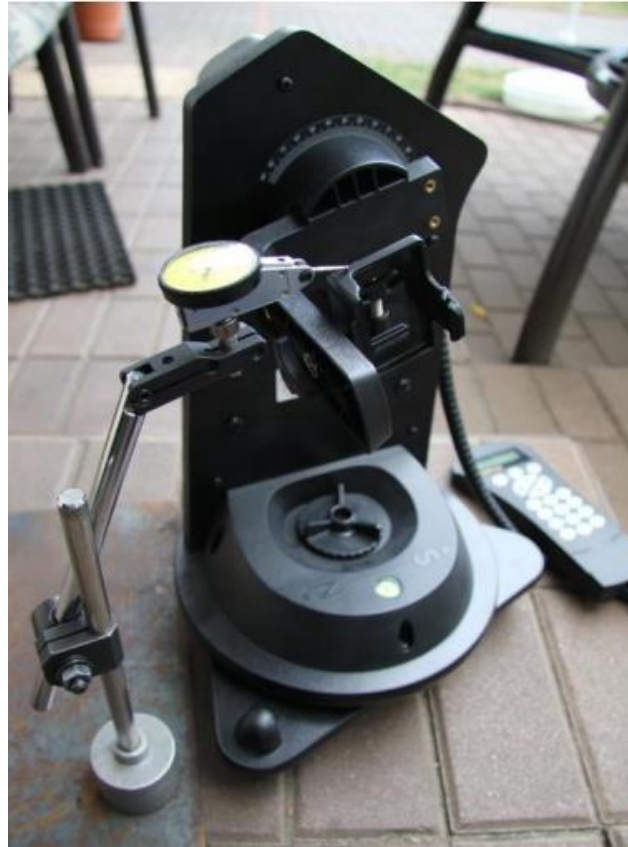
Figure 6. Stand for measuring the repeatability of Skywatcher settings
