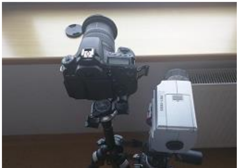
Figure 7. Luminancemeters - matrix and conventional (point measure)
